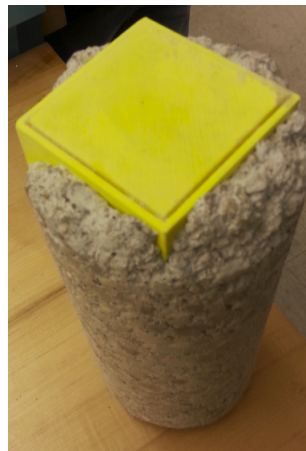
Figure 5: Node encased in concrete after recovery
